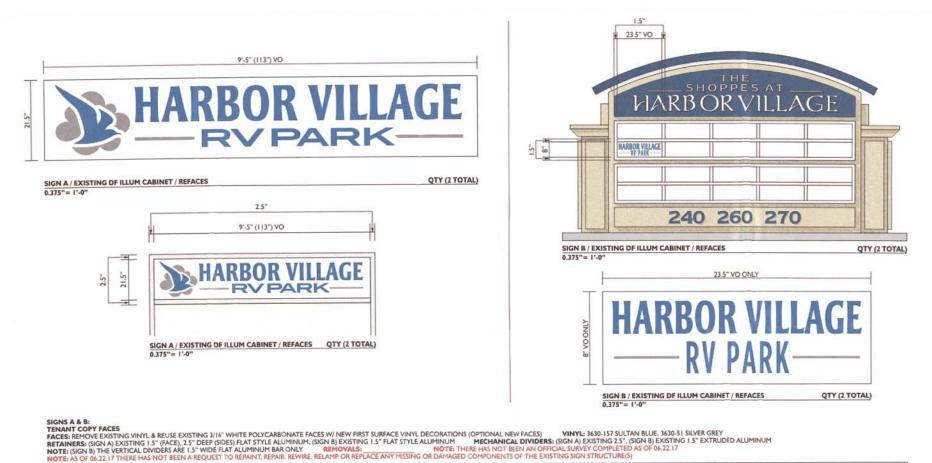
SCOPE OF WORK: FABRICATE & INSTALL (2) TWO NEW FACES FOR EACH SIGN (4 TOTAL FACES)
